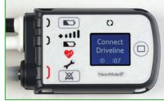
Red Heart Flashing Alarm: This may indicate a Low Flow Hazard. Check patient—the flow may be too low. If patient is hypovolemic, give volume. If patient is in right heart failure—treat per protocol. If the pump has stopped check connections, batteries and controllers as instructed in the section above.
