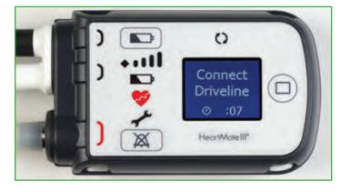
the driveline into the replacement Controller. The pump should restart, if not complete the following steps:
