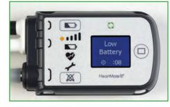
Yellow or Red Battery Alarm: Need to Change Batteries. See changing batteries section on next page.
